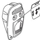
On mufflers without a catalytic converter the screen should be cleaned weekly, or replaced if necessary. On mufflers fitted with a catalytic converter the screen should be checked, and if necessary cleaned, monthly. **If the screen is damaged it should be replaced.**
